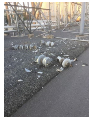
Fig. 9 Example of Storm Damage to AIS Structures Exposed to the Environment
